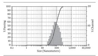
Figure 1. Dynamic Light Scattering Diagram of Distribution of the Size of Nanoencapsulated Essences
