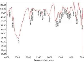
Figure 3. Infrared Spectroscopy of Myristic Acid
