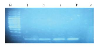
DNA extracted from tissue samples was amplified for  $\beta$ -globulin gene using primers described in methods. Amplification yielded a band of 106 bp. As positive control (P), human DNA from fresh tissue was used; as negative control (N), PCR master mix without DNA was used. Clinical samples, lanes 1 - 3. DNA molecular weight marker, M.
