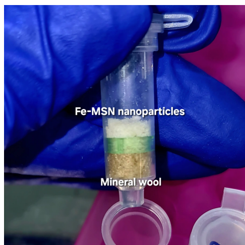
Figure 1. Fe-doped mesoporous silica nanoparticle column (Fe-MSN) extraction column
