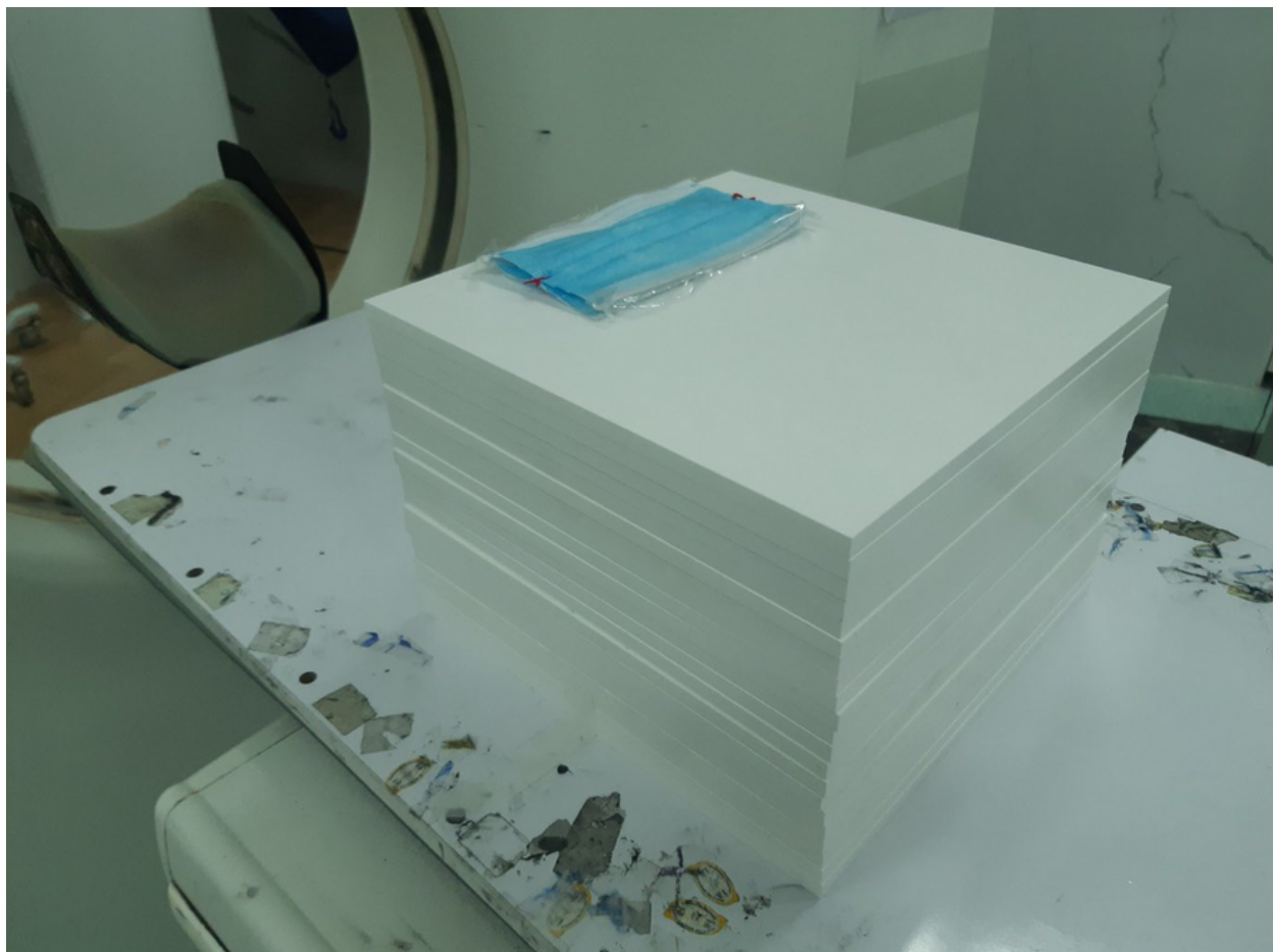
Figure 1. Set up of surgical medical mask (SMM) on polymethyl methacrylate (PMMA) phantom for computed tomography (CT) scan
