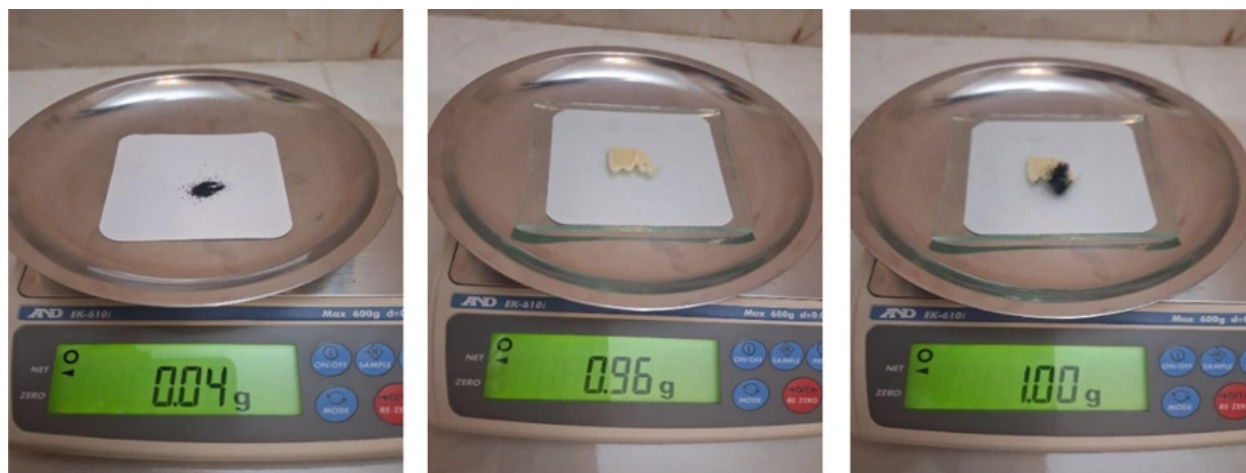
Figure 1. Preparation of 1 g of nanocomposite with a concentration of 4%
